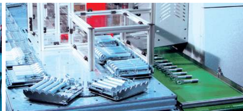
20-station pallet magazine with customer-specific pallets
