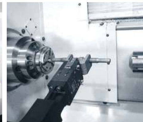
Shaft gripper for automatically loading preformed shafts.
